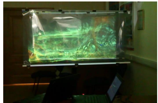
Fig. 2. View of a real mobile demo installation, with dynamic 3D visualization, containing three screens from the perspective of the viewer
